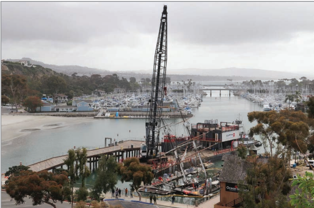
A crane barge lifts the Pilgrim to inspect for damage. Photo by Zach Cavanagh, DP Times .
